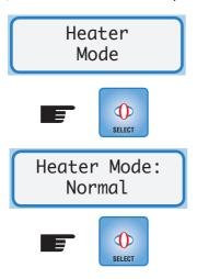
Heater will return to Normal Operation. Pressing Reset will also return the heater to Normal Operation.
