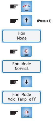
The Fan Mode has been set. Return to Operational Mode by pressing MODE. If the maximum temperature threshold has been exceeded then the Normal Operating Mode shows the fan icon as stationary & no fan speed number.
