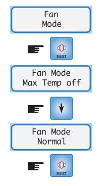
In the 'Normal' setting the fan continue as normal when the ceiling cavity temperature rises above your maximum temperature setting.
