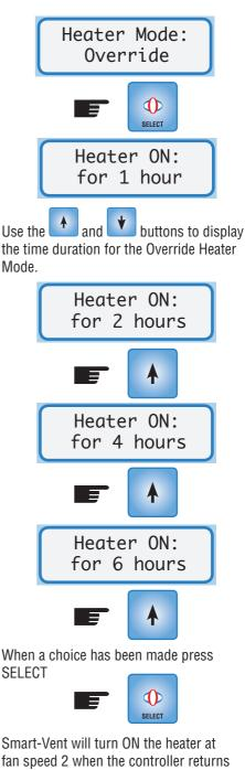
fan speed 2 when the controller returns to Operational Mode. Screen three in Operational Mode will display:
