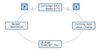
The default screen shows the temperature of the ceiling space and of the room that the
