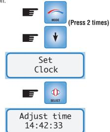
The clock appears in 24 hour format of hours, minutes and seconds. The hours will blink.
