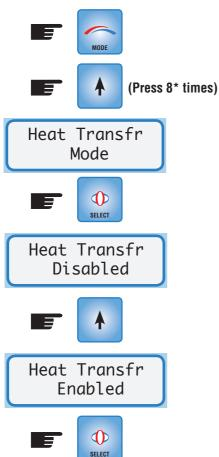
Press 8 times if heater is 'disabled' or 9 times if heater is 'enabled'
