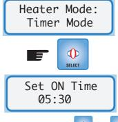
The hours flash. Use the and buttons to set the hour you want the heater to come on. Press SELECT:
