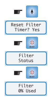
Note: Once the filter timer has been reset the Reset Filter Timer page is removed until the filter is full again. The timer calculates % usage of the filter based on the fan speed.
