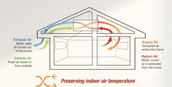
A Heat Recovery System is designed to bring fresh air into your home at a comfortable temperature. These systems recover heat or cooling energy from extracted room air as the heat recovery core transfers the heat from the outgoing air to the incoming air, warming or cooling your home respectively.
