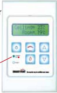
The first line on the display changes from the ceiling temperature to show a 'filter full' message.
